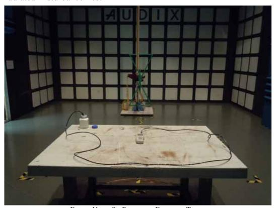
FRONT VIEW OF RADIATED EMISSION TEST
